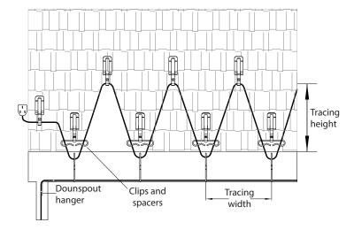
An accurate estimate of the cable length you need is very important because you cannot change the cable length by cutting, splicing or altering it in any way. When calculating cable length, there should be a minimum of 2 inches between the bottom of the drop loop and the bottom of the gutter.
