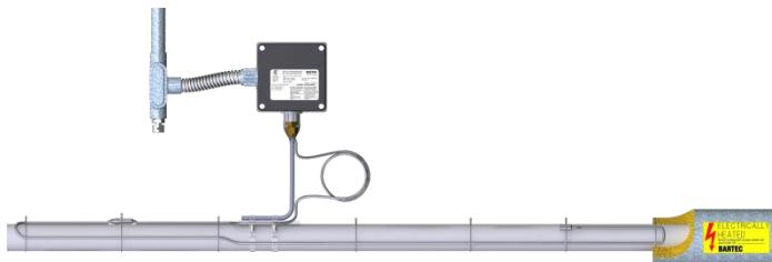
The trace heating system uses a mineral insulated (MI) series resistance trace heater. Its fixed specific resistance offers a constant power output irrespective of the ambient temperature. The alloy 825 or stainless steel outer jacket ensures maximum mechanical strength.
