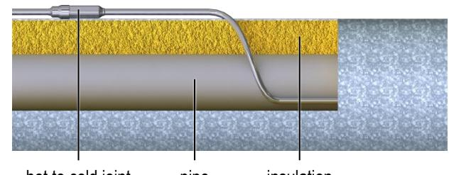
hot to cold joint      pipe      insulation
