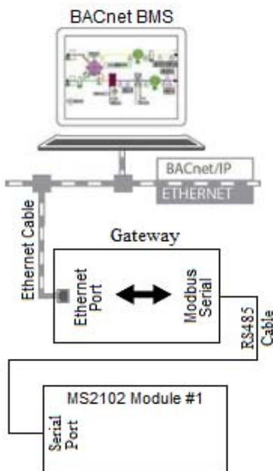
In a MS-2102 heat tracing control module with **BAC**
