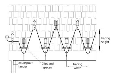
An accurate estimate of the cable length you need is very important because you cannot change the cable length by cutting, splicing or altering it in any way. When calculating cable length, there should be a minimum of 2 inches between the bottom of the drop loop and the bottom of the gutter.
