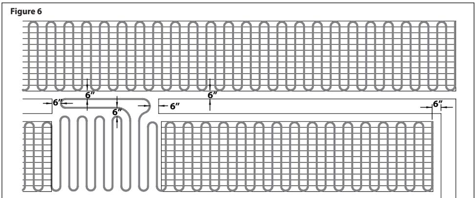
**Note:** It is possible to use adhesive tape ('tuck' tape) to secure the mat or cable onto the subfloor. However, we recommend using the fasteners supplied with the kit to ensure a sturdy installation.
