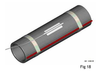
Typical installation of control sensor and sensor for temperature limiting control.
