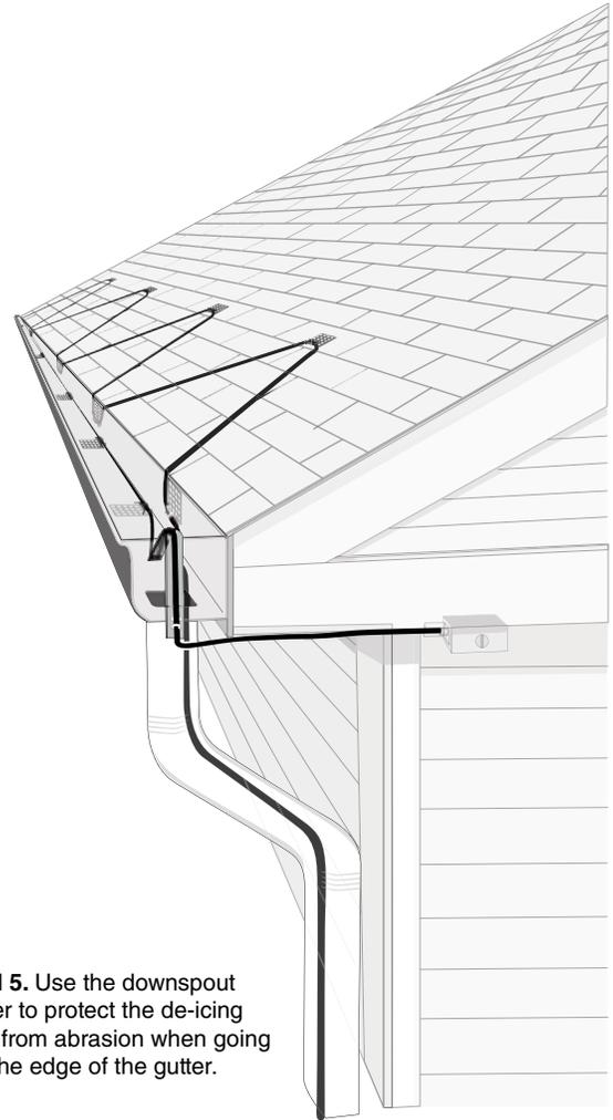
**Detail 5.** Use the downspout hanger to protect the de-icing cable from abrasion when going over the edge of the gutter.
