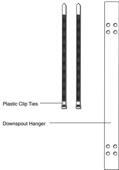
**Detail 1.** Downspout hanger and Plastic Clip Ties.
