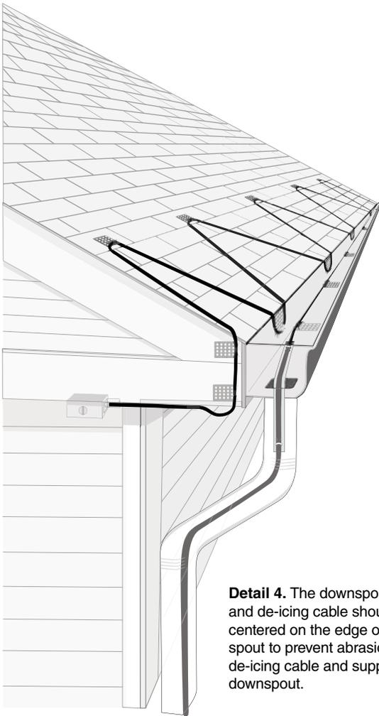
**Detail 4.** The downspout hanger and de-icing cable should be centered on the edge of the downspout to prevent abrasion of the de-icing cable and support it in the downspout.
