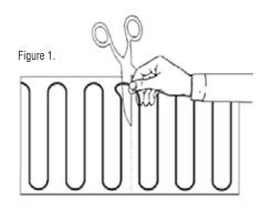
IMPORTANT: Be sure to cut only the mesh. At no time may the heating element wire be cut. This will result in damage to the system.
